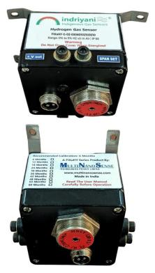
**FIXaHY-G-02-03060102103010** provides a linear output of OV to 5V over the entire range and can be integrated with our single or multi-channel Control & Display Units for local display, trigger-based automation, local alarms, calibration, data logging and system settings.
